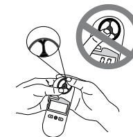
Replacing the Impeller
